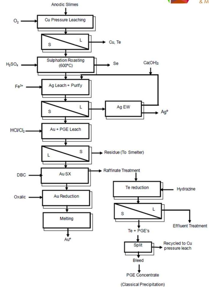
Figure 18. Degussa dm<sup>2</sup> Process to Recover PGE's from Autocatalysts
