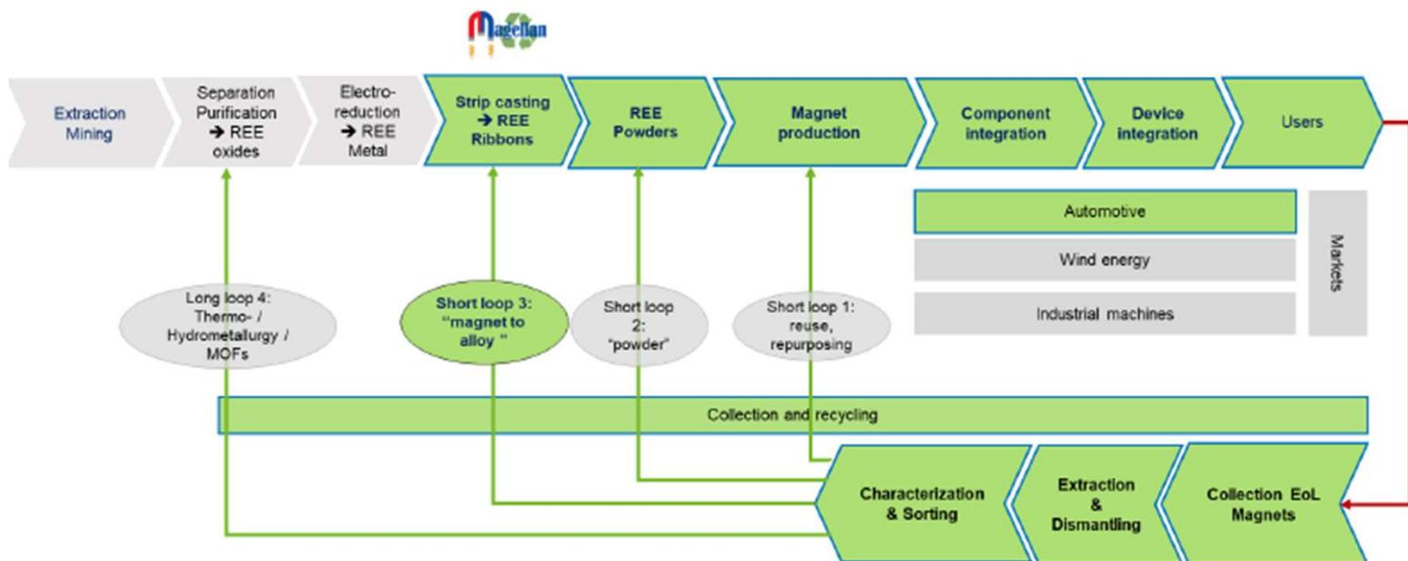
Figure 10 MAGELLAN choice of recycling process: "Magnet-to-alloy"
