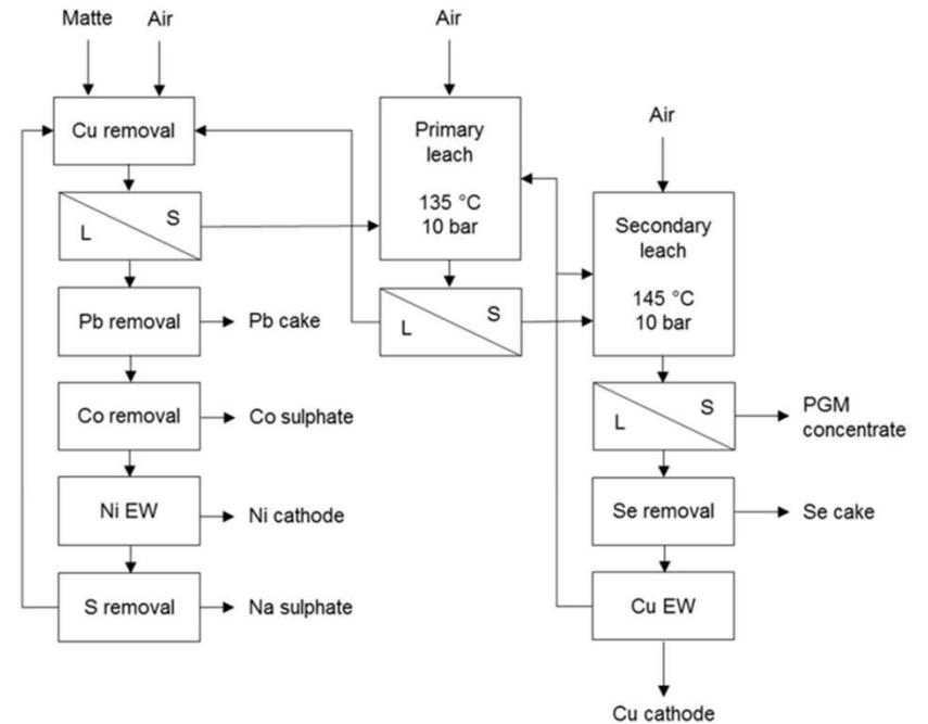
Figure 2. Simplified flow sheet of Rustenburg Base Metals Refinery (adapted from Hofirek & Halton [20]).
